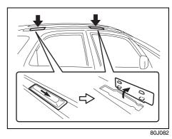
You can use the roof rack anchors to attach the optional roof rack which is available at your SUZUKI dealer. If you use a roof rack, observe the instructions and precautions in this section and provided with the roof rack.
